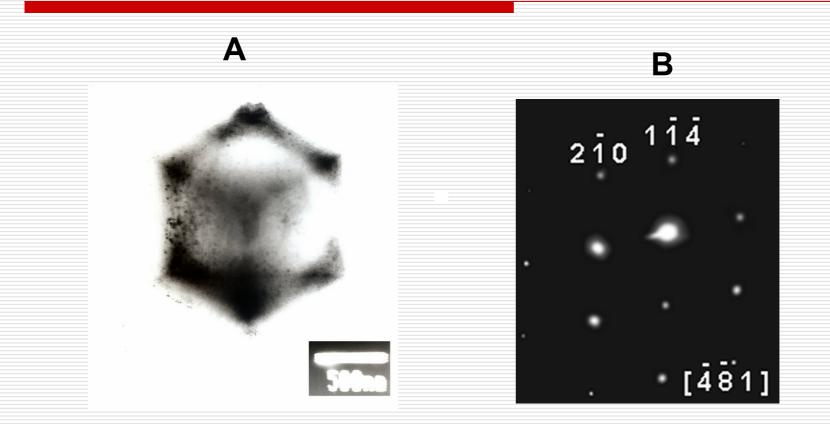
(A) TEM image. (B) diffraction pattern (SAED).  $\rightarrow$  Calcite
