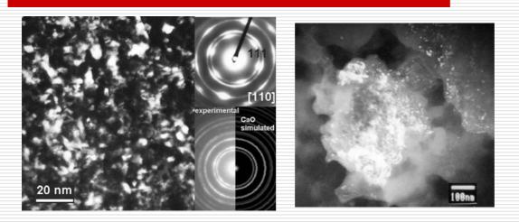
• Decomposition of vaterite phase under the electron beam
