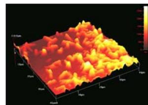
AFM image of adenine crystals grown from solutions on Si wafers. The thickness of the crystals is varied 2 μm for 40 μm long crystals.
