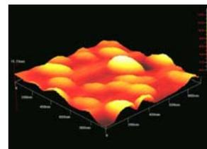
AFM image of adenine crystals following laser etching at 157 nm. The surface roughness was reduced to 5nm following laser illumination at 157 nm with laser fluence of 1 mJ/cm<sup>2</sup> per pulse.
