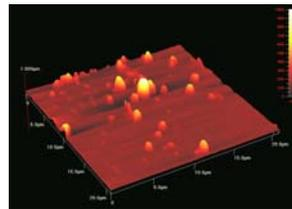
AFM image of adenine crystals following laser etching at 157 nm. The surface roughness was reduced to 30nm following laser illumination at 157 nm with 4000 pulses with the laser fluence of 0.5 mJ/cm<sup>2</sup> per pulse.
