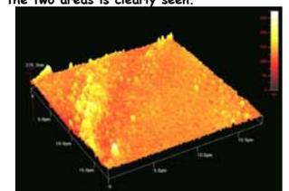
AFM image of non-irradiated and irradiated guanine crystals where the edge (boundary) between the two areas is clearly seen.
