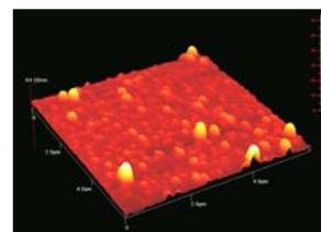
AFM image of adenine crystals following laser etching at 157 nm. The surface roughness was reduced to 1μm following laser illumination at 157 nm with 2000 pulses with the laser fluence of 0.05 mJ/cm<sup>2</sup> per pulse. The etching rate of the crystal was 0.5 nm for a laser fluence of 1mJ/cm<sup>2</sup>.
