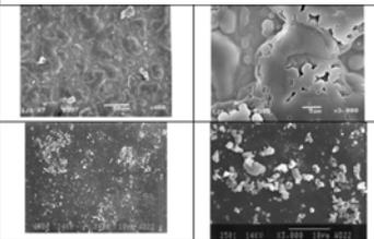
SEM images of guanine crystals grown from solutions on Si wafers. Crystals were grown at different shapes depending on the experimental conditions.
