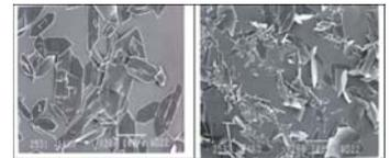
SEM images of non-irradiated (left) and irradiated (right) cytosine crystals. When the laser fluence exceeds the threshold value of 2 mJ/cm<sup>2</sup>, the crystal collapses due to induced stress from the laser pulse which destroys the thermo dynamical equilibrium of the crystal.
