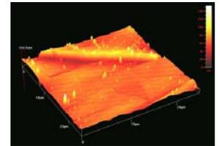
AFM image of non-irradiated and irradiated cytosine crystals where the edge between the two areas is clearly seen.
