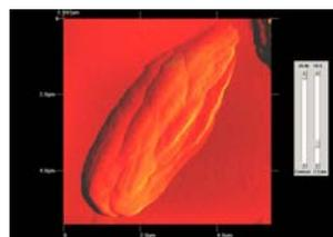
AFM image of adenine crystal. Long adenine crystals are formed from agglomerations of such crystals.
