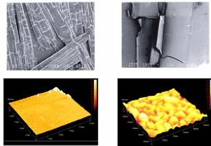
AFM and SEM surface morphology images of cytosine crystals grown from solutions on Si wafers. Crystals were grown at a variety of shapes depending on the experimental conditions.
