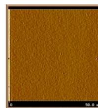
Surface image of the S3 copolymer in contact mode. The image was taken with scan size of 8,92 x 8,92 μm. The surface RMS roughness was 0.3 nm.
