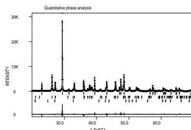
Rietveld plot ( $R_{wp} = 11$ ). Experimental (crosses), calculated (solid line) and difference (solid line below) Vertical bars denote  $\text{CuK}\alpha_1$ ,  $\theta_2$  reflection positions of calcite (top row), aragonite (middle row) and vaterite (lower row).
