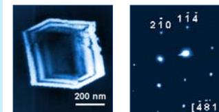
TEM image and a diffraction pattern of Calcite
