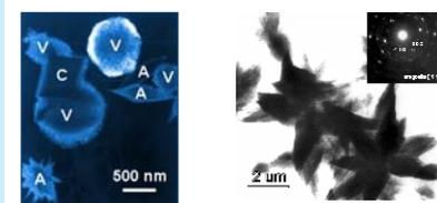
TEM image of different  $\text{CaCO}_3$  crystals and a diffraction pattern of Aragonite
