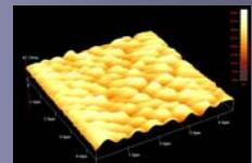
3D-AFM images of the edge between exposed and non exposed areas in Teflon at 157 nm.
