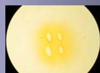
Micro-array of PTFEMA spots , fabricated at 157 nm by surface laser ablation in PTFEMA. The dimensions of each one of the oval shaped spot was 10 X 20 μm.
