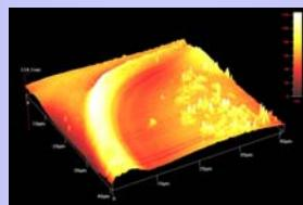
Surface dipping from volume ablation. At lower laser fluence, the pressure is not high enough to support surface swelling and the dissociated photo-fragments escape from defects within the volume to the surface. As material is constantly removing the illuminated volume collapses with a 40 nm dipping. The area was illuminated with 100 laser pulses, having 100 μm laser spot-size at 1 mJ/cm<sup>2</sup> for each pulse.
