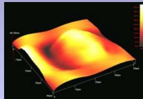
When the pressure is not high enough to ablate the polymer volume, surface swelling is taking place as is clearly seen in the AFM image. The surface swells ~50 nm. Around the edges surface dipping can be clearly seen. The surface was illuminated with 100 laser pulse of 10 μm spot size at 1 mJ/cm<sup>2</sup>.
