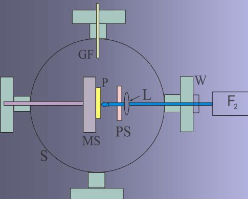
❖ Experimental set up for 157 nm laser surface treatment of biopolymers. F<sub>2</sub>: 157 nm laser. MS: X-Y-Z-θ computer controlled stage. S: Stainless-steel chamber. PS: Optical projection system. P: Polymeric thin films. L: Focusing CaF<sub>2</sub> projection system. W: CaF<sub>2</sub> window.
