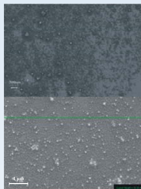
SEM images of micelle like structures in PS-P2VP/ FeCl_3 hybrid film following chemical reduction. The average dimension of nano particles is 30nm.
