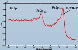
XPS spectrum of the Fe 2p peak obtained after 20 minutes of sputtering on the SVP film.
