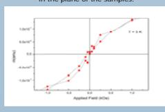
The magnetization curve versus applied field, of the VUV reduced S2VP/Fe films at 5K. The applied magnetic field is lying in the plane of the samples.
