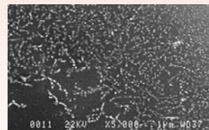
SEM image of the S2VP loaded with FeCl<sub>3</sub> and SmCl<sub>3</sub> precursors on Si/Ta substrates following chemical reduction.
