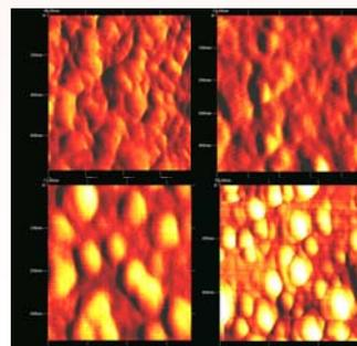
AFM images of the S2VP loaded with FeCl<sub>3</sub> and SmCl<sub>3</sub> precursors on Si/Ta substrates following VUV laser reduction.
