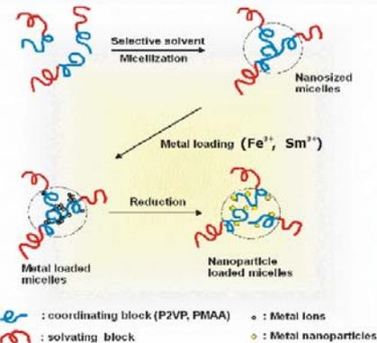
Schematic lay out of the reduction process catalyzed by wet chemistry. The last step can be also realized by VUV light illumination at 157 nm of the preformed thin films.
