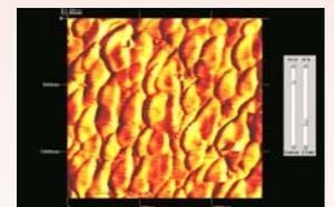
AFM image of the S2VP loaded with FeCl<sub>3</sub> and SmCl<sub>3</sub> precursors on Si/Ta substrates and following VUV laser reduction.
