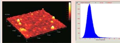
AFM image of the S2VP loaded with FeCl<sub>3</sub> and SmCl<sub>3</sub> precursors on Si/Ta substrates following chemical reduction. The height histogram of the S2VP film following loading of the FeCl<sub>3</sub> and SmCl<sub>3</sub>.
