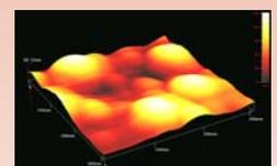
At higher magnification micelles with size scaled down to the ~ 50 nm can be seen.
