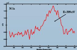
XPS spectrum of the N 1s peak obtained after 20 minutes of sputtering on the SVP film.
