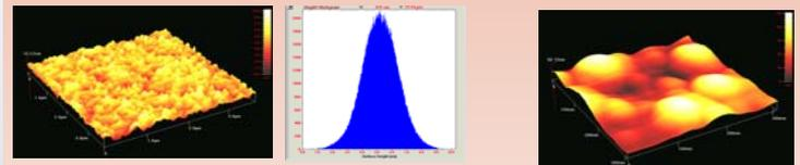
AFM image of the surface morphology of the S2VP film prior loading the precursors. The height histogram (Z-direction) of the S2VP film prior loading the precursors.
