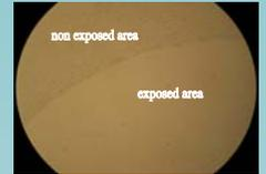
Optical images of spin coated Teflon AF solutions of less than 6% concentration (FC75 solvent) results, in locally nonuniform (rough) films in the non exposed area.
