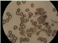
Monolayer aggregation of Ulocladium sp spores grown on Si substrate. The average length of the spores was 10 μm.
